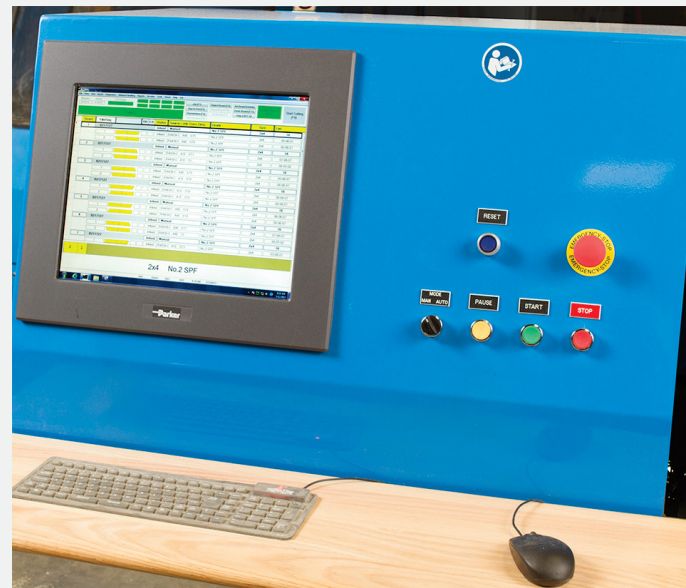
Operator Control Panel
